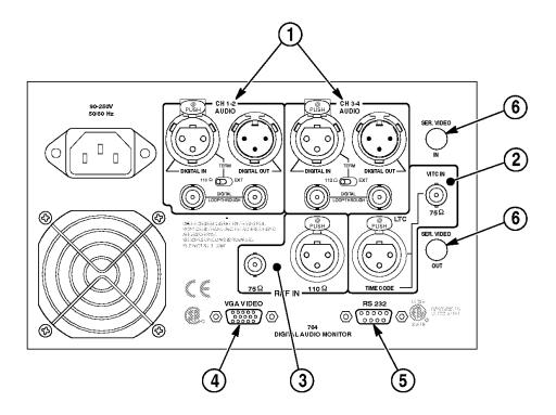
Figure 3: The 764 rear panel and connectors
